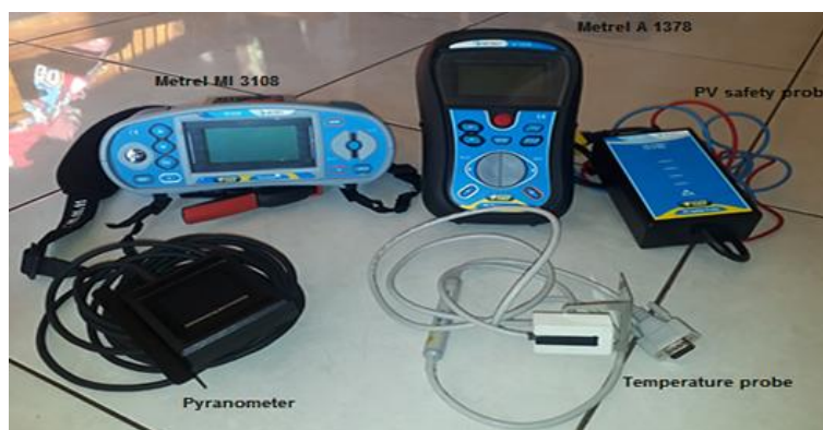
Gambar 4. Metrel MI 3108 Eurotest PV dan Metrel A 1378 PV remote unit
